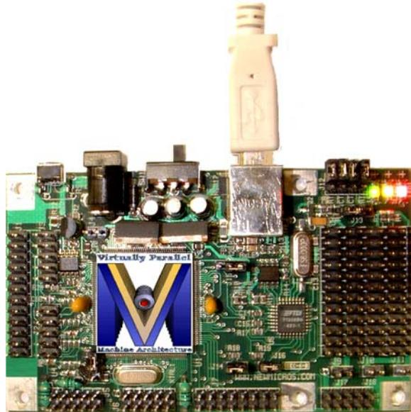
Connect the provided USB (A to B type) cable from the PC to the ServoPod-USB™. All three LED's should come on within a short delay after the USB cable is plugged in. If the LED's don't come on after more than a few seconds, unplug the USB cable quickly. Please see the trouble shooting section of this manual or contact NMI technical support for help, before going any further.
