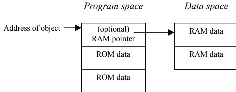
Note that although `OBJECT` creates a pointer to Program space, it does not reserve *any* Program or Data memory. That is the responsibility of the programmer. This is done in the same manner as the `<BUILDS` clause of a `<BUILDS DOES>` definition, using `P,` or `PALLOT` to add cells to Program space and `,` or `ALLOT` to add cells to Data space. The programmer can use `OBJECT` to build a custom defining word for each class. See the example below.
