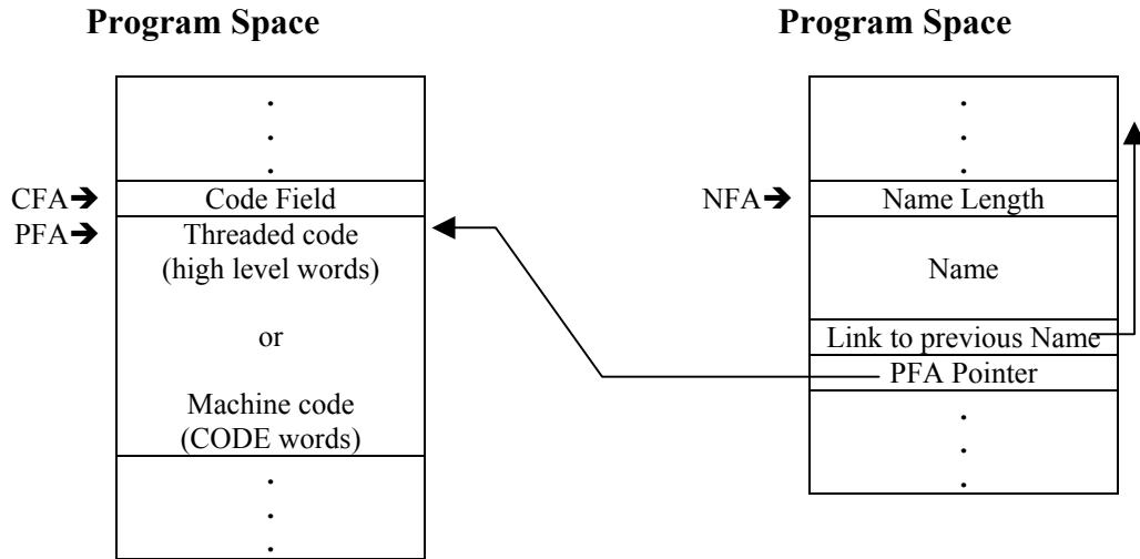
If you have not enabled separated heads, the words you add to the dictionary will have the header immediately before the executable body.
