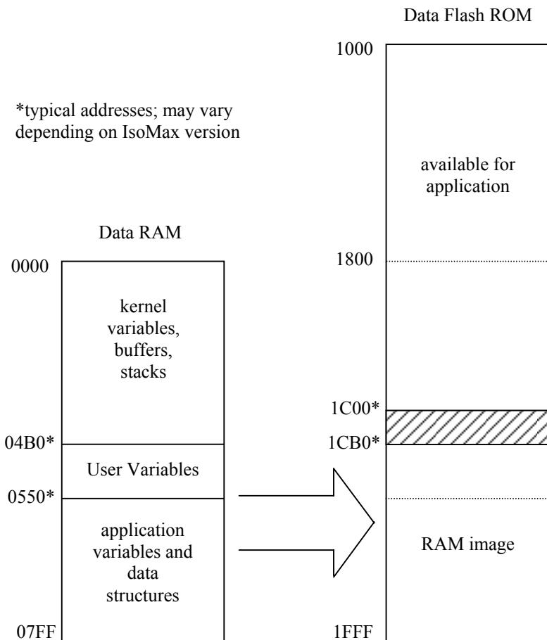
Kernel buffers include the stacks, working “registers,” and other scratch data that are used by the IsoMax interpreter. These are considered “volatile” and are always cleared when the IsoPod is powered up. These are also private to IsoMax and not available to you.
