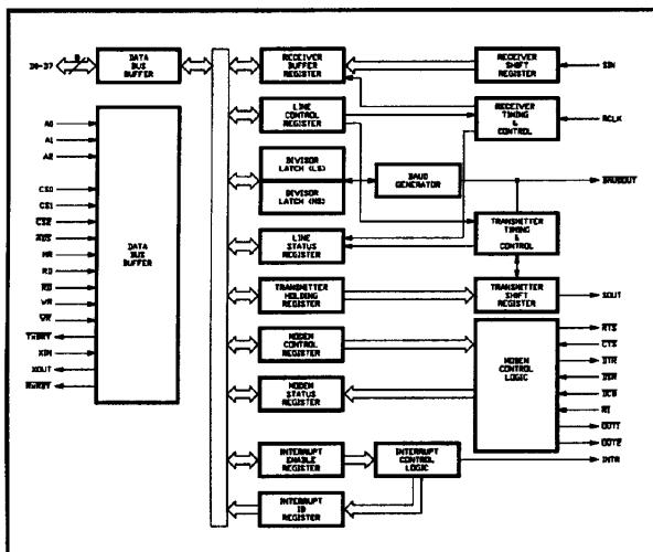
The **UART** has an internal baud rate generator that is capable of dividing the timing reference clock input by divisors of 1 to  $(2^{16}-1)$ , and producing a 16x clock for driving the internal transmitter logic. The crystal determines the baud rates. It is normally a 1.8432 MHz crystal for selection of baud rates up to 19,200 baud.
